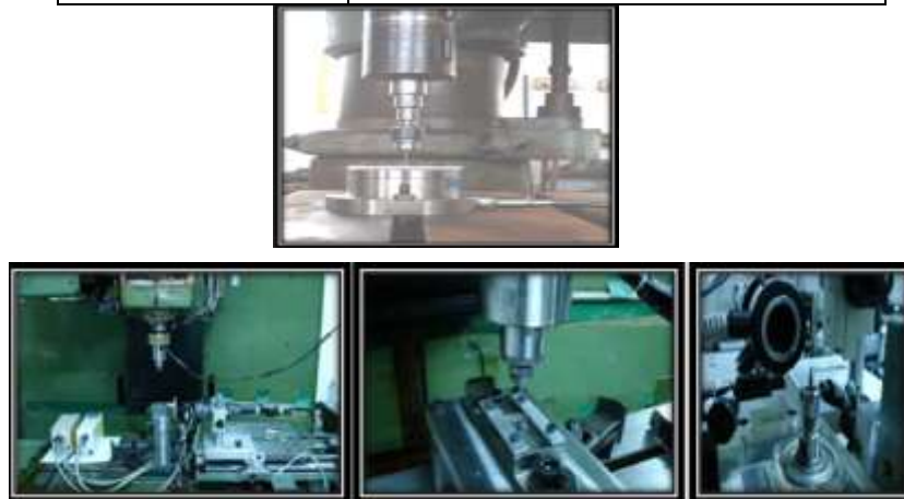
Figure 3.1: (Top) Micro-drilling machine and machine vision unit, (Bottom) Air spindle and work piece fixture & Illumination and measurement unit.
