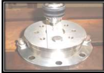
Fig 3.2: Dynamometer, Work piece set up
